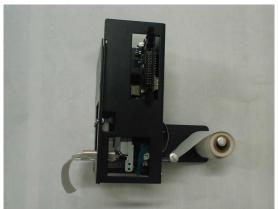
Figure P3: AC7074 Printer – Side View, Showing Proper Roll Placement
