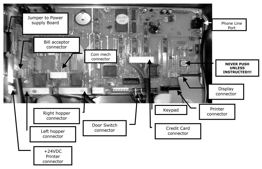
Figure 9 – AC8060.2 Main Logic Board
